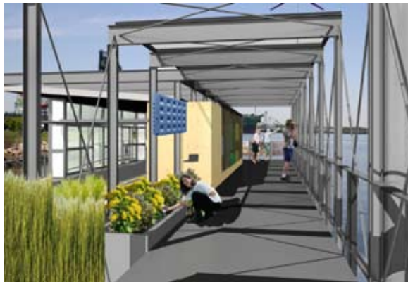
Native plants purify rainwater used onboard before release into the Elizabeth River.
